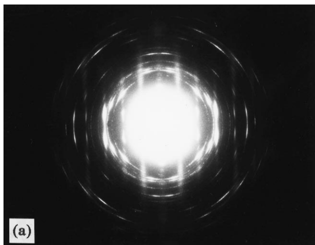
Figure 9 (a) BF electron micrograph and (b) the corresponding electron diffraction pattern of HDPE-iPP double-layered films, which were heat-treated at 150°C for 10 min, and then isothermally crystallized at 126°C for 5 h. The chain direction of the oriented iPP substrate is indicated by the arrow
